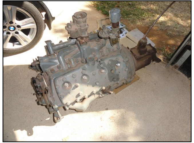
Ford engine 1938 V8 flathead 24 stud
